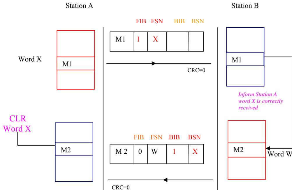
For a forward message any value of FIB can be given (0 or 1). If this message is correctly received the value of the BIB is to be same as FIB. For the above example FSN=X, FIB=1, If it is received correctly by B then it transmits BIB=1, BSN=X to station A.
