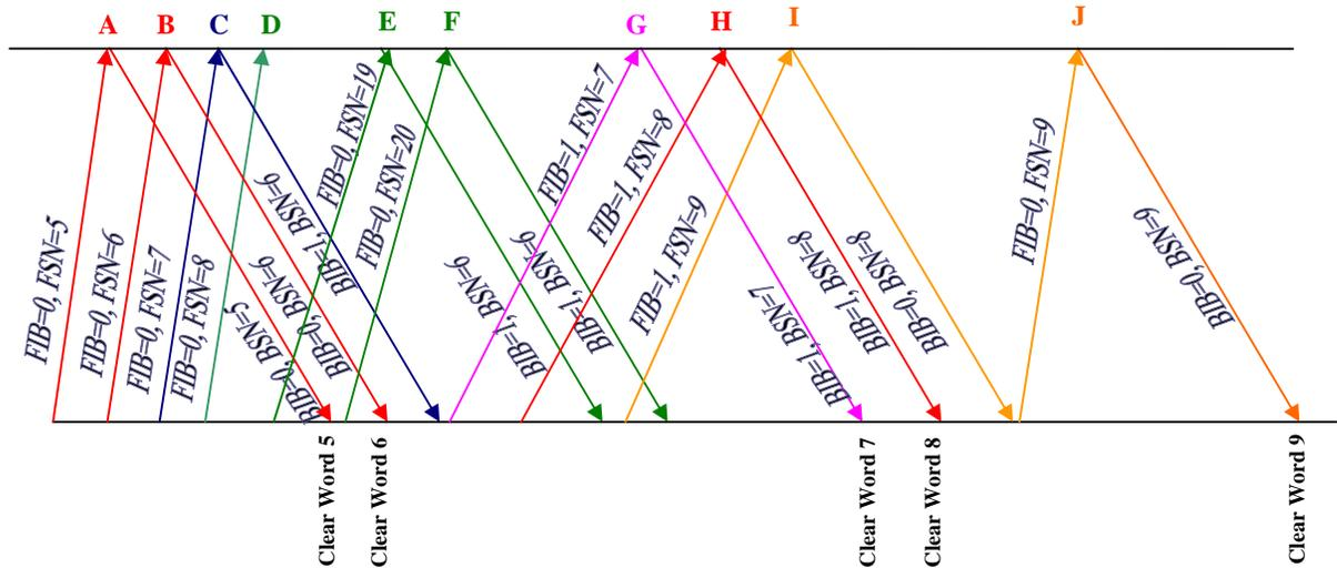
The above timing chart shows how messages are exchanged between two stations. A to J are highlighted incidents in this message transactions. The following are observed.
