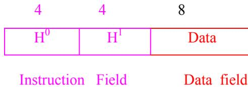
There are two headers in the instruction field.  $H^0$  and  $H^1$  each header has 4 bits. The length of data field varies according to  $H^0$  and  $H^1$  from 0 to about 60 octets.
