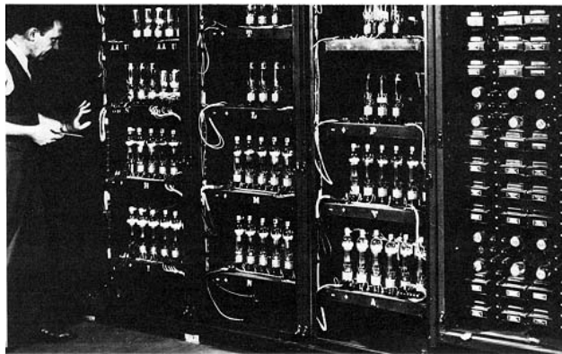
ENIAC Rear view (note vacuum tubes).
