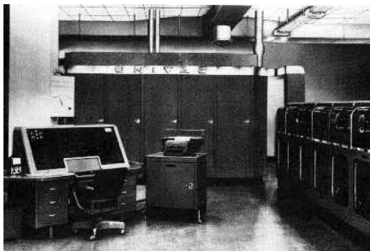
The First General-Purpose Computer for Commercial Use : Universal Automatic Computer (UNIVAC).
