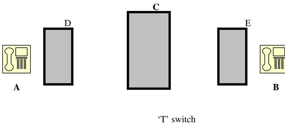
C is the Master Switch, where as D and E are Remote Switches. Each remote switch will connect to Master Switch by 16 PCM systems namely  $P_0$  to  $P_{31}$ . A is speaking with B on  $P_0$  TS8, where as B is speaking to A on  $P_{18}$  TS20.
