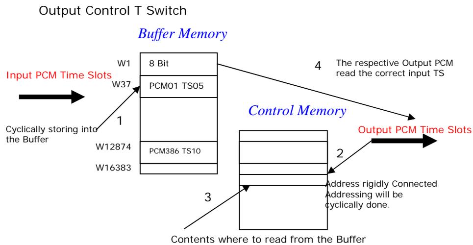
In the Control memory word number 37 will be addressed by  $PCM01_b TS05$  and the contents is to read the Buffer memory in the word number 12874. Similarly word number 12874 is addressed by the  $PCM386_b TS10$  and the contents of the control memory is to read word number 37. The size of the control memory is 14 bit word and 16384 words. The Processor deployed to carry out the instructions of the switching equation given above should have cycle time better than  $(125/512) * 30 * 2 \mu s$ .
