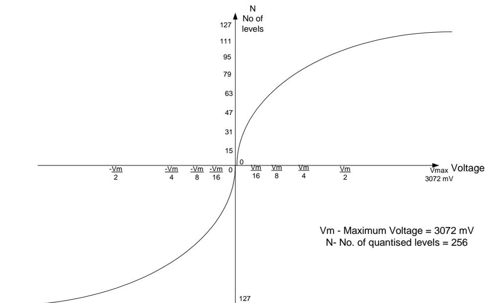
1.4 Each quantized level will be converted to binary before transporting the quantized level (related to the sample) into the transmission media. Assuming a telephone will generate a maximum of  $\pm 3072$  mV calculate the encoded format that will be sent in the transmission media for the following sample values.
