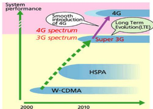
Long Term Evolution (LTE) will be the next technologies for mobile broadband service which capable to have potential bandwidth up to 100 Mbps for downloading and 50 Mbps for uploading. Long Term Evolution (LTE) is a 4G wireless broadband technology as the next generation of 3G which designed to increase the capability, speed of mobile broadband network and its performance. Long Term Evolution (LTE) is developed by the Third Generation Partnership Project (3GPP)
